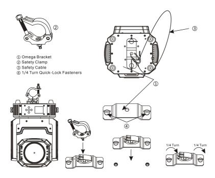
Regardless of the rigging option you choose for your QBEAM 50, always be sure to secure your fixture with a safety cable. The fixture provides a built-in rigging point for a safety cable on the hanging bracket as illustrated above. Be sure to only use the designated rigging point for the safety cable and never secure a safety cable to a carrying handle.
