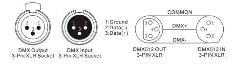
For installations where the DMX cable has to run a long distance or is in an electrically noisy environment, such as in a discotheque, it is recommended to use a DMX terminator. This helps in preventing corruption of the digital control signal by electrical noise. The DMX terminator is simply an XLR plug with a 120  $\Omega$  resistor connected between pins 2 and 3, which is then plugged into the output XLR socket of the last fixture in the chain. Please see illustrations below.
