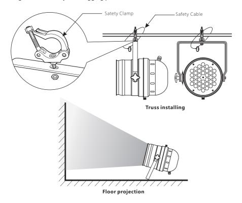
Regardless of the rigging option you choose for your LEDPAR 64, always be sure to secure your fixture with a safety cable. The fixture provides a built-in rigging point for a safety cable on the hanging bracket as illustrated above. Be sure to only use the designated rigging point for the safety cable and never secure a safety cable to a carrying handle.
