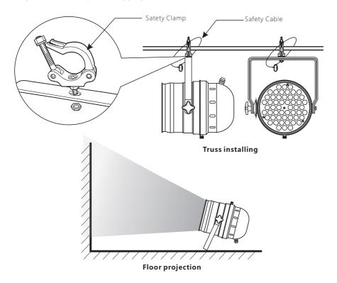
Regardless of the rigging option you choose for your LEDPAR 64, always be sure to secure your fixture with a safety cable. The fixture provides a built-in rigging point for a safety cable on the hanging bracket as illustrated above. Be sure to only use the designated rigging point for the safety cable and never secure a safety cable to a carrying handle.
