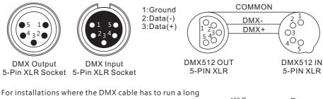
distance or is in an electrically noisy environment, such as in a discothegue, it is recommended to use a DMX terminator. This helps in preventing corruption of the digital control signal by electrical noise. The DMX terminator is simply an XLR plug with a 120  $\Omega$  resistor connected between pins 2 and 3, which is then plugged into the output XLR socket of the last fixture in the chain. Please see illustrations below.
