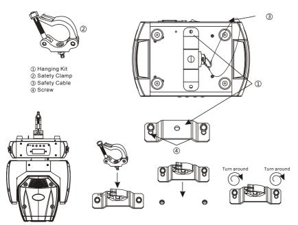
Regardless of the rigging option you choose for your MINISPOT 90, always be sure to secure your fixture with a safety cable. The fixture provides a built-in rigging point for a safety cable on the hanging bracket as illustrated above. Be sure to only use the designated rigging point for the safety cable and never secure a safety cable to a carrying handle.
