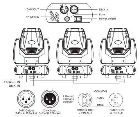
For installations where the DMX cable has to run a long distance or is in an electrically noisy environment, such as in a discotheque, it is recommended to use a DMX terminator. This helps in preventing corruption of the digital control signal by electrical noise. The DMX terminator is simply an XLR plug with a  $120\ \Omega$  resistor connected between pins 2 and 3,which is then plugged into the output XLR socket of the last fixture in the chain. Please see illustrations below.
