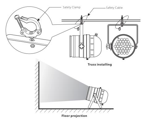
Regardless of the rigging option you choose for your LEDPAR 64UV, always be sure to secure your fixture with a safety cable. The fixture provides a built-in rigging point for a safety cable on the hanging bracket as illustrated above. Be sure to only use the designated rigging point for the safety cable and never secure a safety cable to a carrying handle.
